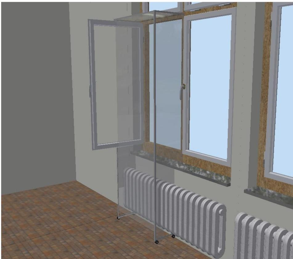
**Figure 2:** CAD model of a movable (rollable) draught projection system built of polycarbonate double-webbed sheets, aluminium corner profiles, and furniture casters for historic-building-preservation, draught-reduction and the thermally comfortable introduction of fresh air from a window to the floor (via fully or partially opened turn-only window or laterally tilted window). The window remains fully functional and can be closed outside lesson time so that no additional heat loss occurs.
