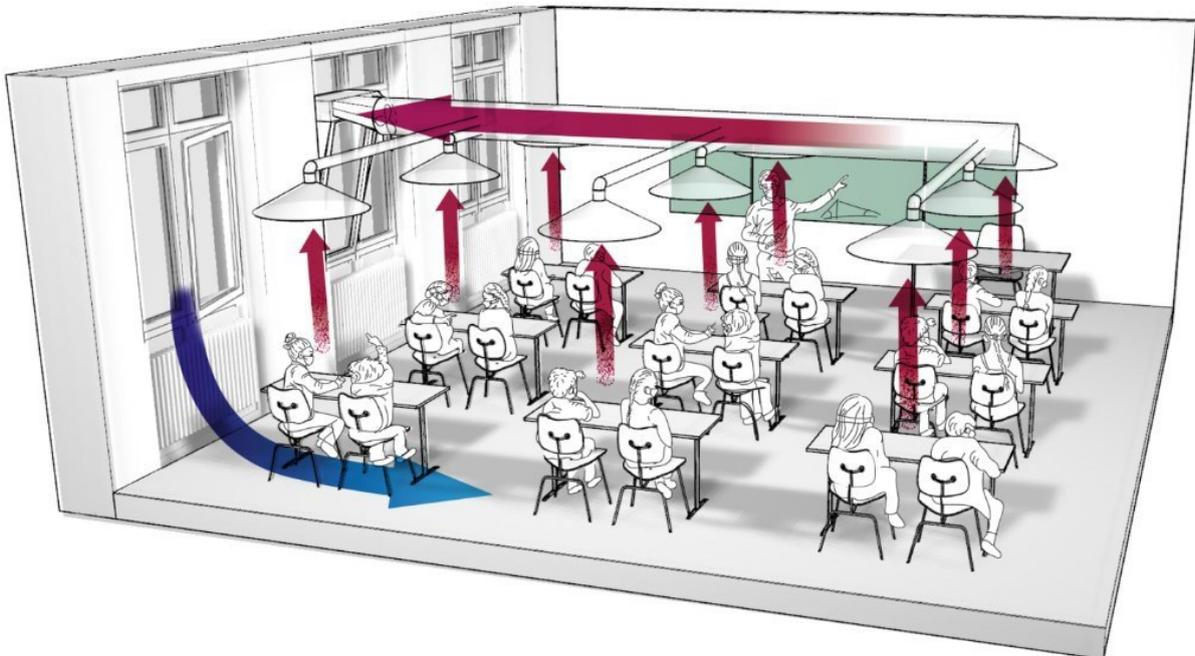
**Figure 4:** Schematic diagram of a mechanical extract ventilation system with distributed extract ducts and hoods (MPIC-MEV hood version) (ventilation-mainz.de).
