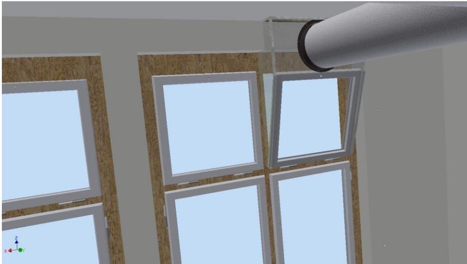
**Figure 1:** CAD model of a ventilator box built from polycarbonate double web panels and aluminium corner profiles suitable for conservation-protection and the thermally-insulated connection of the extractor fan to a bottom-hung window. The window remains fully functional and can be closed via the existing OL90 control system outside of class time so that there is no additional heat loss.
