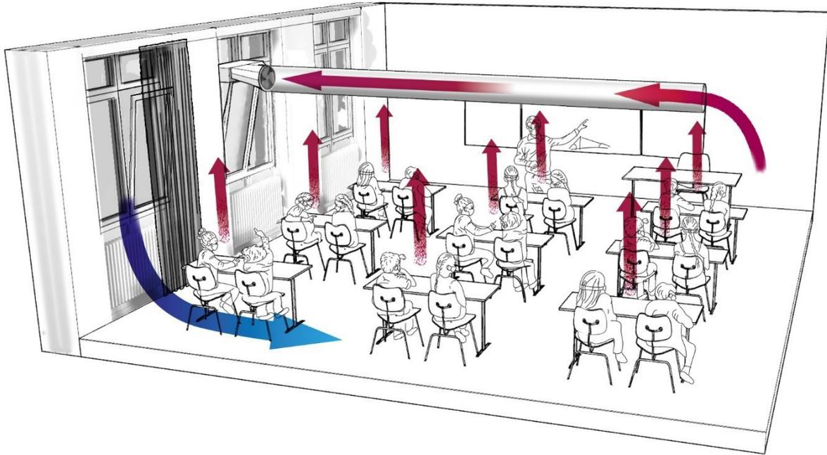
**Figure 3:** Schematic diagram of a mechanical extract ventilation system with central extract duct (MPIC-MEV base version) (ventilation-mainz.de).
