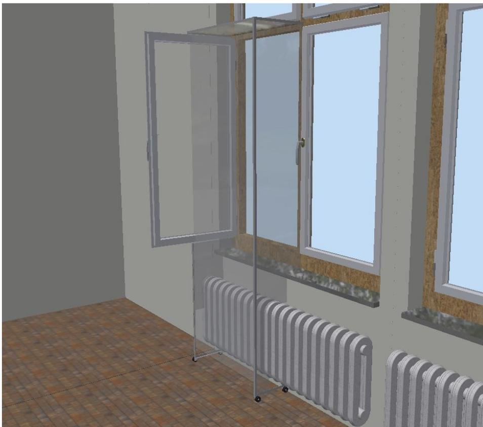
**Figure 2:** CAD model of a movable (rollable) projection built of polycarbonate double-webbed sheets, aluminum corner profiles, and furniture casters for monument-protection-, heat-protection-, and comfort-compatible introduction of fresh air from a window to the floor (fully or partially opened turn-only window or laterally pivoted window). The window remains fully functional and can be closed outside lesson time so that no additional heat loss occurs.
