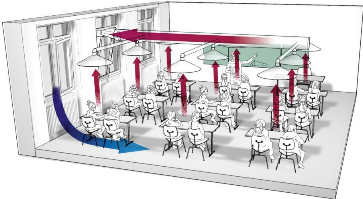
**Figure 4:** Schematic diagram of a fan-assisted window ventilation system with distributed extraction hoods (Mainz model – basic version) (ventilation-mainz.de).
