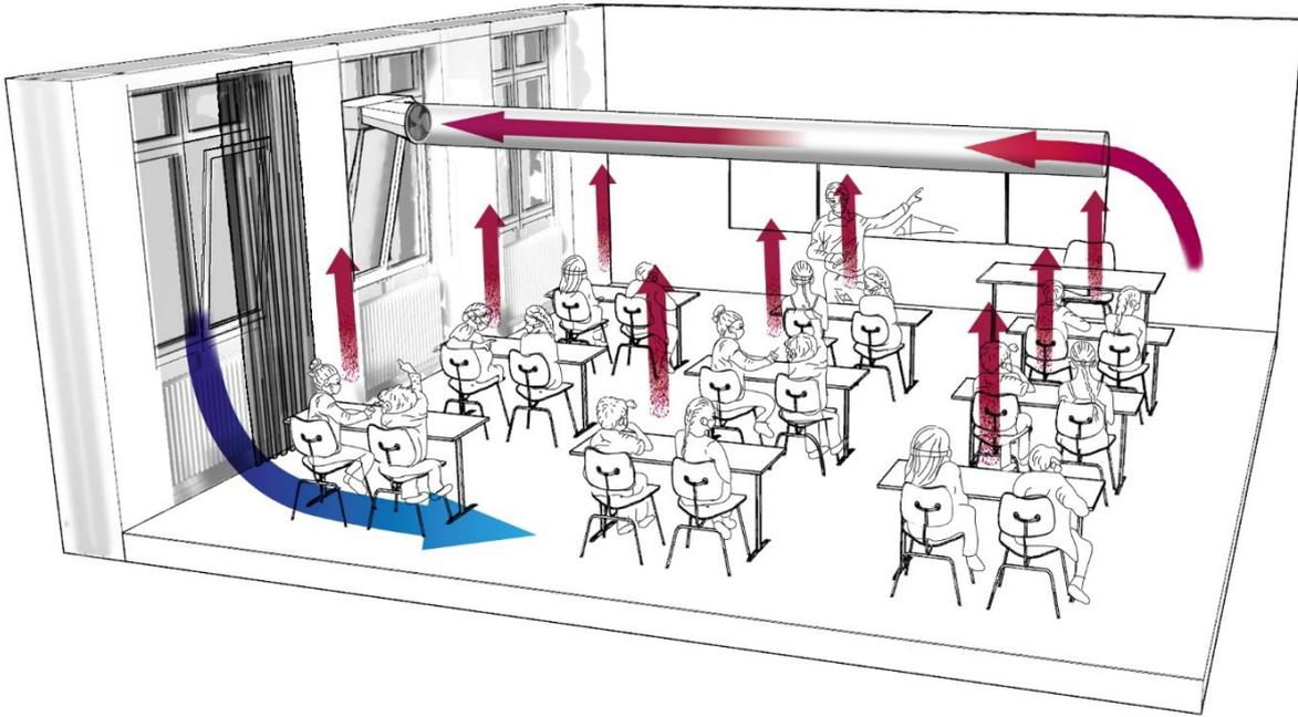
**Figure 3:** Schematic diagram of a fan-assisted window ventilation system with exhaust duct (Mainz model – basic version) (ventilation-mainz.de).
