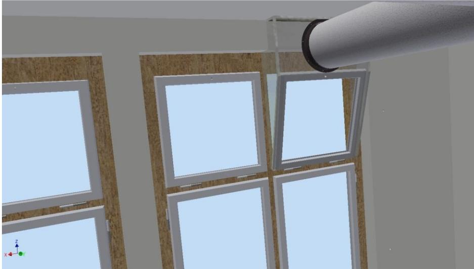
**Figure 1:** CAD model of a ventilator box built from polycarbonate double web panels and aluminum corner profiles for monument-protection- and thermal-insulation-compatible connection of the extractor fan to a laterally pivoted window. The window remains fully functional and can be closed via the existing OL90 remote control outside of class time so that there is no additional heat loss.
